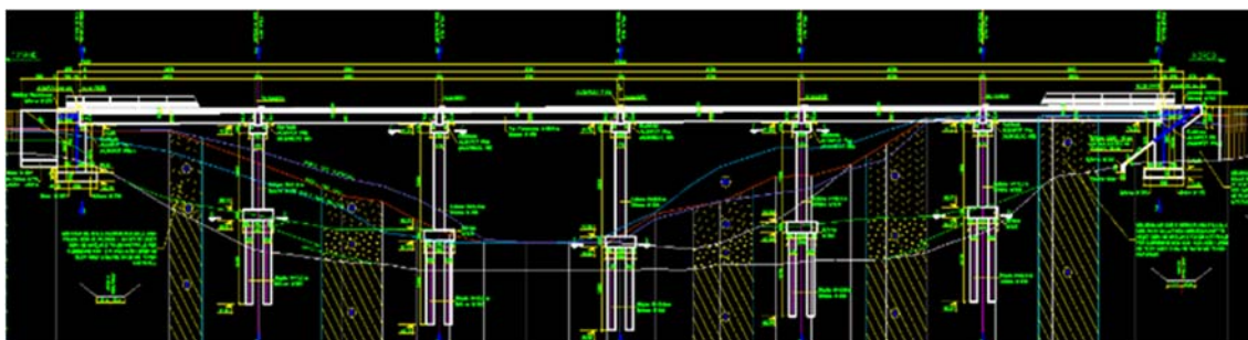
Technical design of New bridge over the Erzeni River at km 3+233.97 – longitudinal cross section
